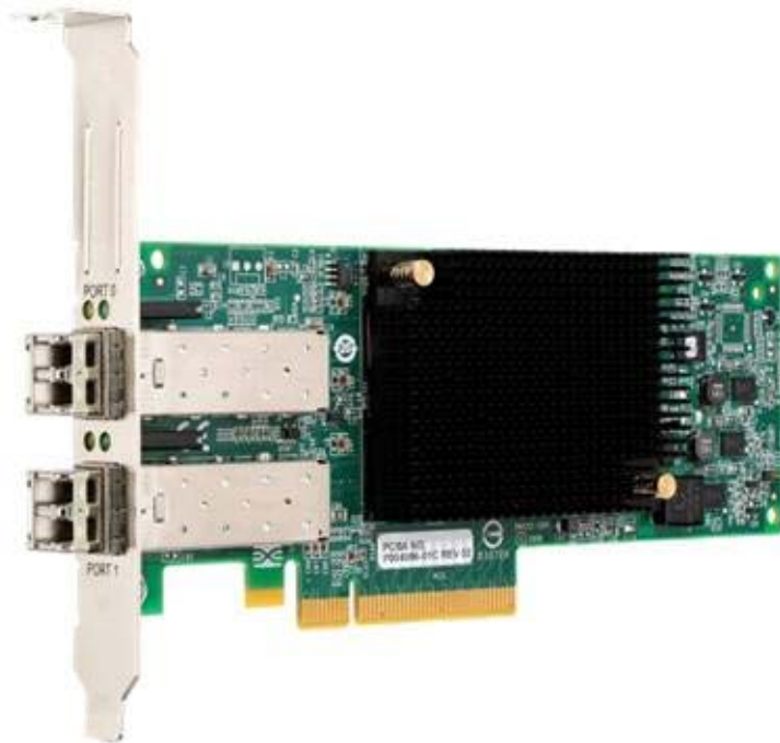
Figure 1. Emulex 10Gb Virtual Fabric Adapter for IBM System x (with optional SFP+ transceivers installed)
